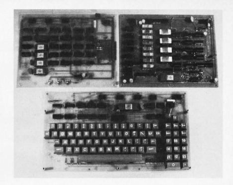
Photo 2: Here are the three main boards of the Sphere system. At the upper left is the video interface board with 512 bytes of memory used for the display. At upper right is the main processor board with the 6800, 4 KB of dynamic memory and 1 KB of EROM. The lower board is the keyboard assembly, which includes a numerical keypad and cursor control keys as well as a full alphanumeric keyboard.
