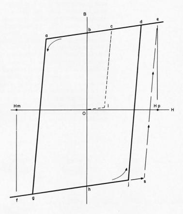
Figure 3: Memory properties are derived from the hysteresis properties of the core material. When the applied H value is 0, the residual B value in the core material will depend upon the past history of magnetization. This figure and subsequent figures show the magnitude of the vector quantities H and B, with positive and negative values corresponding to the two directions of rotation about the core axis.
