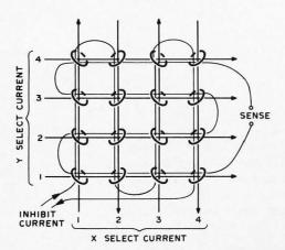
Figure 9: The inhibit line is added to the array assembly of cores so that it is possible to avoid changing the state of a given core with coincident current selection.
