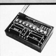
Pictured above is the new OP-80A High Speed Paper Tape Reader from OAE. This unit has no moving parts, will read punched tape as fast as you can pull it through (0-5,000 c.p.s.), and costs only \$74.50 KIT, \$95.00 ASSEMBLED & TESTED. It includes a precision optical sensor array, high speed data buffers, and all required handshake logic to interface with any uP parallel I/O port.
