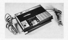
Uses the industry standard tape saturation method to beat all FSK systems ten to one. No modems or FSK decoders required. Loads 8K of memory in 17 seconds. This recorder, using high grade audio cassettes, enables you to back up your computer by loading and dumping programs and data fast as you go, thus enabling you to get by with less memory. Can be software controlled.
