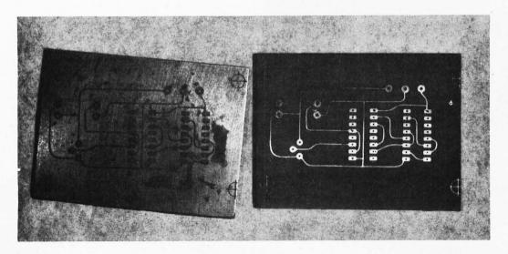
Photo 3: Results of Exposure. After being exposed, the photosensitive layer is developed, using an appropriate solution. An etch resist pattern will then remain on the board as in the example at left. (The dark blotches are oxidation on the copper.) The board is then etched with the usual ferric chloride solution. The finished product (hopefully free of imperfections) is a printed circuit board such as the one at right.
