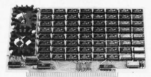
PLUG DIRECTLY INTO 8800 or 8800 BOARD COMPATIBLE SYSTEM • TURNS OFF YOUR WAIT LED (8080 RUNS AT FULL SPEED) • LESS THAN 520 nS ACCESS AND CYCLE TIME • LOW POWER (LESS THAN 225 mA/1K at 5 VOLTS) • 100% NEW INDUSTRIAL COMPONENTS • EASY INTERFACE TO HOME BREW • 50/50 GOLD PLATED EDGE CONTACTS • EPOXY BOARD WITH PLATED THRU HOLES • 8K or 4K WITH EXPANSION • SOCKET PROGRAM 4K or 8K ADDRESS SLOT • DETAILED ASSEMBLY AND THEORY
