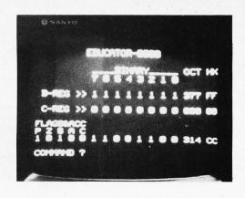
Photo 3: To illustrate the use of hexadecimal immediate values, this photo shows the operation of XRI H'C3'.
