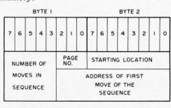
Figure 3: Primary and Subchain Pointer Formats. The pointer tables are composed of two byte elements which contain information on the number of moves required, and the address of the first move of the sequence.
