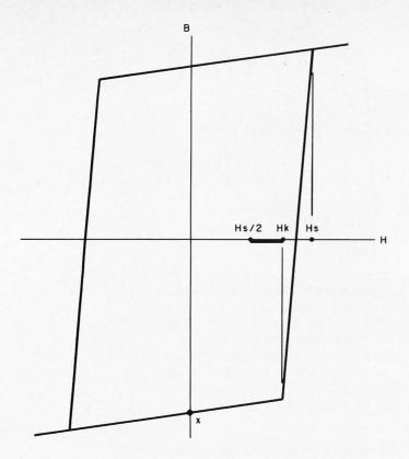
Figure 8: The half-select current i/2 must generate an H field less than Hk if a change of state is to be avoided. Similarly, the full select current of i must generate an H field strength greater than Hs to ensure switching. This leaves a range of field strengths (and corresponding current values) from Hs/2 to Hk which introduces a critical tolerance for the select currents in a core memory design.
