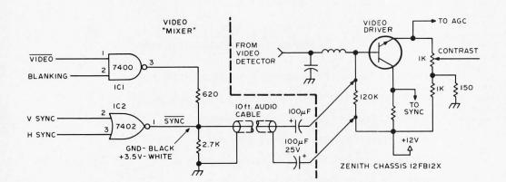
Figure 1: The "Ignorance Is Bliss" Television Drive Circuit. The components to the left of the dashed line were added as part of the interface. The components to the right of the dashed line are part of the Zenith 12FB12X chassis which was used for the television display.
