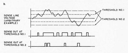
Figure 14: Sense Amplifier. The purpose of the sense amplifier is to create an output signal which can be strobed into a TTL latch at the appropriate moment, given the signals induced into the sense wire of the memory. For testing, the thresholds are set using the variable resistance of 200 ohms in a voltage divider from the +5 volt supply.
