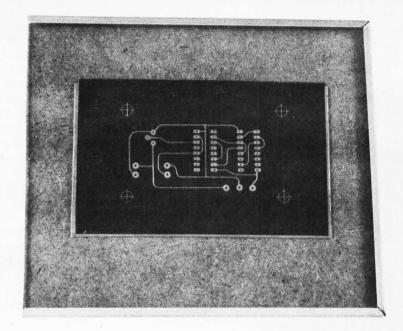
Photo 2: Printing the Circuit. Once a negative of the artwork has been created, the next step is to print the circuit. The negative is placed over a sensitized PC board and held firmly in place by a alass cover plate in the printing frame, The glass guarantees smooth and even contact for accurate transfer of the image. The board is then exposed to a photoflood lamp for one to three minutes.
