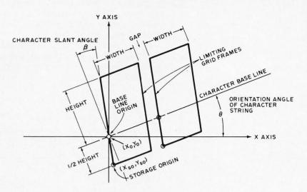
Figure 5: Character Orientation. To add an element of finesse to the plotting function, provision for general purpose rotation and slanting is a desirable feature. There are two angles to specify: angle  $\theta$  is the orientation angle of the baseline for a character string; angle  $\beta$  is the frame slant relative to a perpendicular through the base line.
