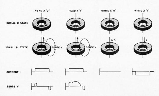
Figure 5: Using the physics of core switching. This figure shows the four basic operations needed to manipulate the binary state of a memory core: Read a "0", read a "1", write a "0" and write a "1".
