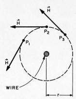
Figure 1: For a wire carrying current i directed out of the page, the magnetic field  $\mathbf{H}$  is proportional to i/r. The direction of  $\mathbf{H}$  is tangential to the circle of radius r, as shown for points  $P_1$ ,  $P_2$  and  $P_3$ .
