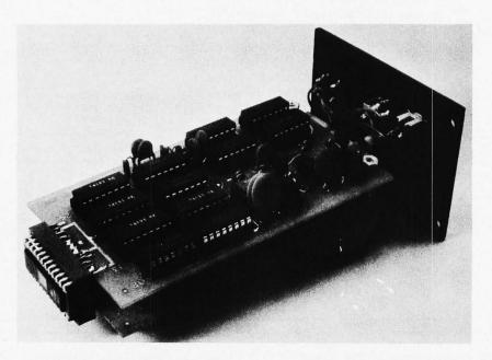
Photo 1: The Solid State Sales Video Camera Kit, as assembled. The kit includes the two printed circuit boards and all electronic parts, but does not include the packaging into a neat box with lenses, etc. The charge coupled device sensor is shown mounted between the two boards in this photograph.
